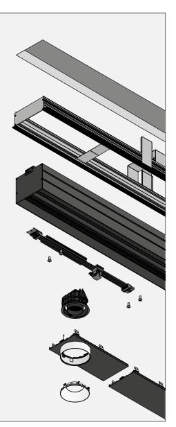
Schematic representation of assembly Holon 120 single in-Cana: profile + luminaire + louvre
