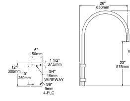
WMA12 Note: Back plate is welded to the arm.
