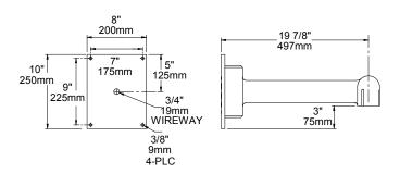
WMA20 Note: Back plate is welded to the arm.
