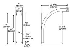
WMA24 Note: Back plate is welded to the arm.
