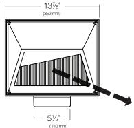
Arrows indicate main thrust of light distribution, in elevation.
