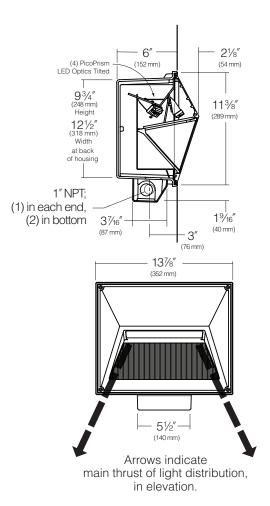
**Housing and Junction Box:** Die-cast, low-copper (<0.6% Cu) aluminum to prevent corrosion when cast in concrete. Junction box shall have an internally removable cover, a volume of 25 cu in., and four 1" NPT conduit taps. Two taps in the bottom and one in each end, all with removable plugs. Housing and junction box further protected for permanence by a clear anodize coating. Cover furnished to keep the housing clean until the electrical components are installed.
