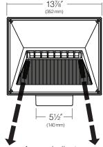
Arrows indicate main thrust of light distribution, in elevation.
