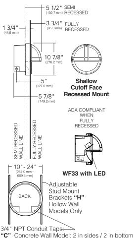
"C" Concrete Wall Model: 2 in sides / 2 in bottom
