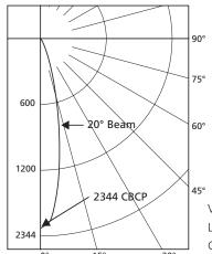
Voltage: 120 Watts: 6.84 Amps: 0.83 Lumens: 470 CBCP: 2344 Beam: 20° CCT: 3000K Efficacy: 69 Lm/W
