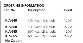
**NOTE:** Output wattage is not to exceed 25 amps on each circuit. Weather conditions must be considered when determining load on transformers, hot weather areas should reduce the output wattage to prevent heat build-up on circuit breakers. The voltage at each fixture must not exceed 12 volt. Load and distance must be considered when determining which voltage tap to use. A good maintenance program is required to replace lamps as they burn out to prevent over-voltage of remaining lamps.
