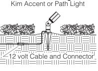
**Cable Installed In-grade**
