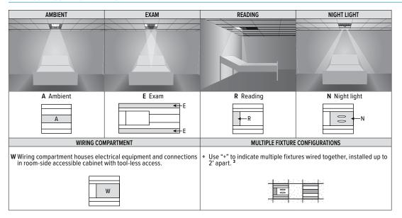
Some fixture configurations do not allow all drivers to be located within the night light or wiring compartment. Drivers and electrical connections will be located in primary fixture or wiring compartment (when "W" or "+" is specified) as space allows.
