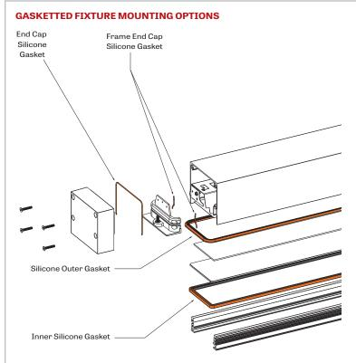
Lens and enclosure are sealed with inner and outer silicone gaskets
