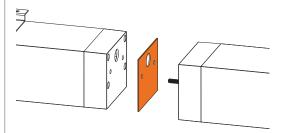
All individual sections are joined together onsite using the  $\frac{1}{4}$ "-20 screws and nuts provided. The joint between 2 adjacent individual sections is sealed by a silicone gasket attached to one of the 2 sections. The electrical connection between sections is made through the holes provided in the end-caps.
