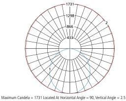
— 1 - Vertical Plane Through Horizontal Angles (90-270) (Through Max. Cd.)
