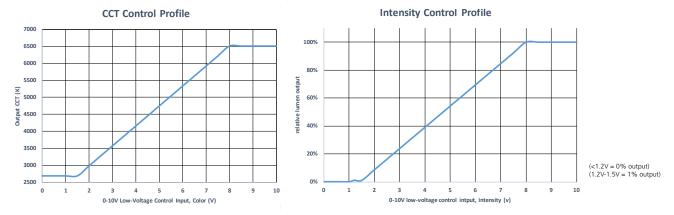
NOTE: The provided information is the typical expected performance of a single luminaire. Additional luminaires on the same 0-10V line may result in different control profiles. Fine tuning of system performance should be completed after installation is complete. To avoid CCT shift between luminaires, care should be taken to minimize voltage drop on the CCT Control line. It is recommended to limit the load on the CCT control circuit to twenty (20) 45T or ten (10) 67T/90T luminaires or less.
