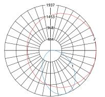
Maximum Candela = 1937 Located At Horizontal Angle = 0, Vertical Angle = 20
