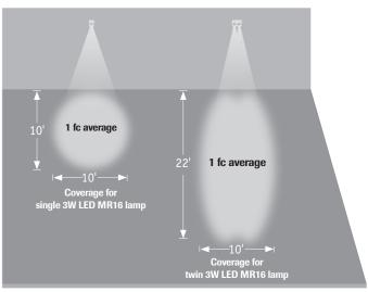
Meets Life Safety Code minimum illuminance of 0.1 fc and average illuminance of 1.0 fc. Assumes open space with no obstructions, mounting height of 7.5', ceiling height of 9' and reflectances of 80/50/20. Photometry files available on the Dual-Lite web site (www.dual-lite.com).
