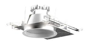
**Installation:** Adjustable Bar hangers included. Universal adjustable mounting brackets also accept 1/2" EMT conduit or 11/2" or 3/4" lathing channel (by others) or Prescolite 24" bar hangers (B24 or B6).
