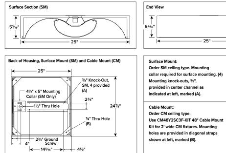
For Cable Mount a 2" x 3" access plate with (4) 7/8" KOs provided in place of Mounting Collar shown.
