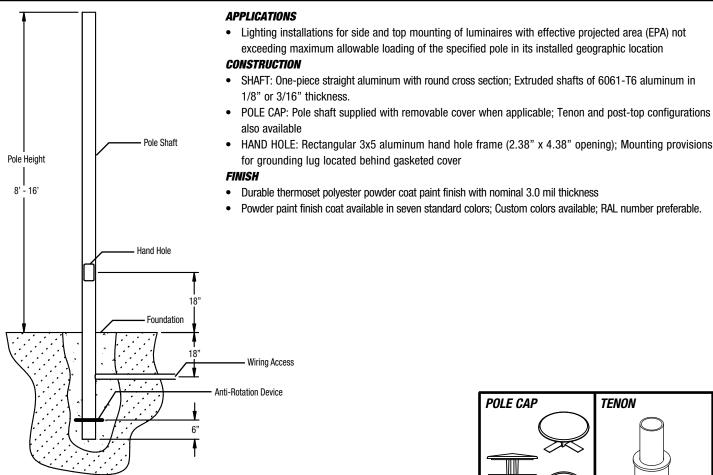
\*Local civil engineer should be consulted for proper foundation design
