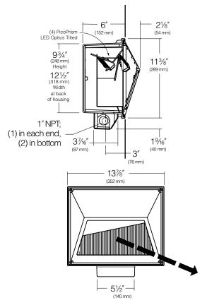
Arrows indicate main thrust of light distribution, in elevation.
