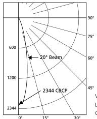
Voltage: 12 Watts: 6.84 Amps: 0.83 Lumens: 470 CBCP: 2344 Beam: 20° CCT: 3000K Efficacy: 69 Lm/W
