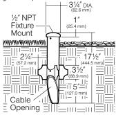
• Low Voltage Spear Mount: Die-cast low copper aluminum with K" NPSM fixture mount. Stainless steel set screw locks fixture into mount. Cable slot allows easy fixture mounting before or after installation in ground. Super TGIC powder coat paint over clear anodizing and titanated zirconium conversion coating.
