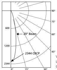
Voltage: 12 Watts: 6.84 Amps: 0.83 Lumens: 470 CBCP: 2344 Beam: 20°
