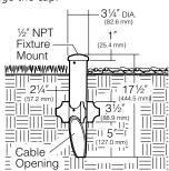
• KLV400 Low Voltage Spear Mount: Die-cast low copper aluminum with 1/2" NPSM fixture mount. Stainless steel set screw locks fixture into mount. Cable slot allows easy fixture mounting before or after installation in ground. Super TGIC powder coat paint over clear anodizing and titanated zirconium conversion coating.
