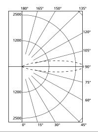
Voltage: 12 Watts: 6.8 Amps: 0.83 Lumens: 445 CBCP: 2226 Beam: 20° CCT: 3000K Efficacy: 65 Lm/W
