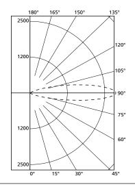
Amps: 0.816 Voltage: 12 Watts: 6.77 Lumens: 460 CBCP: 2264 Beam: 20° Lm/W CCT: 3000K Efficacy: 68
