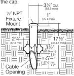
• KLV400 Low Voltage Spear Mount: Die-cast low copper aluminum with 1/2" NPSM fixture mount. Stainless steel set screw locks fixture into mount. Cable slot allows easy fixture mounting before or after installation in ground. Super TGIC powder coat paint over clear anodizing and titanated zirconium conversion coating.
