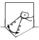
Internal LED tray adjusted up to 30 degrees for aiming.
