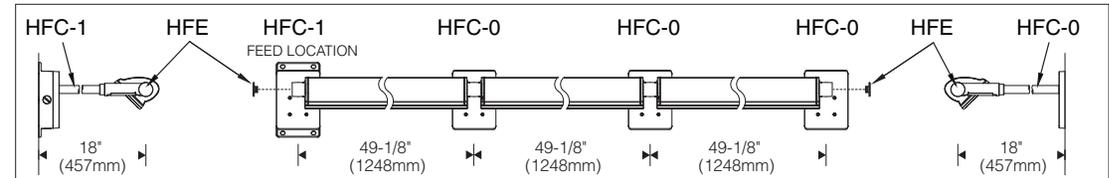
**EXAMPLE 2:** 12ft row with (3) 4ft S175 fixtures and (4) 18" wall wash cantilevers, recessed outlet box at second hanger. Order (3) S175-R04\_ fixtures, (4) HFC-0 surface hangers (one to use recessed outlet box feed), and (1) HFE end kit.
