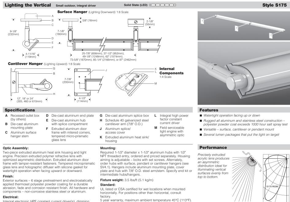
Integral electronic HPF constant current driver(s), dimming drivers are optional. For complete driver specifications, see website, reference document <u>MA-1303</u>. 84" leads exit one end of housing.
