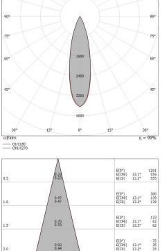
E(0°) E(C90) E(C0) 1.16 2.5 E(C90) E(C90) E(C0) 1.40 1.41 3.0 Distance [m] Cone diameter [m C0/C180 (Half-peak divergence: 26.4°) C90/C270 (Half-peak divergence: 26.2°)
