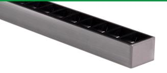
The VERS Louver is designed to eliminate glare, rendering more precise light distribution. A custom-sized black VERS louver fits snugly above a low-profile clear or diffused lens to mitigate diode imaging and glare issues. Metal endcaps combined with the flush louver and extruded aluminum VERS housing provide a sleek compact fixture.
