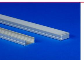
The WIDE LED extrusion is Q-Tran's widest profile extrusion, making it able to fit even our widest LEDs: RGBW. It is available in satin, black, and bronze finishes and is offered in three different lenses; clear, polar, and diffused. With a clear lens, its light transmission is 97 degrees. WIDE can be configured with in-fed wires, back-fed wires, and wires from the left and right for both lead and exit, giving you more freedom with your design. Available in lengths up to 98.43".
