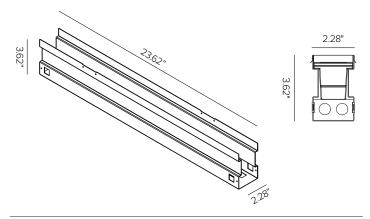
MINI MERCURE aluminum installation sleeve, supplied with 2ea removable end caps. Complete with internal supports for installations in concrete, single or continuous row applications.
