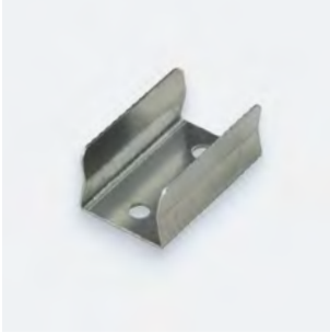
KKCP-02 (1no.) KKCP-52 (500no.) Clip (allow 3 per metre/40in) S/Steel finish L25/W16.7/H15.5mm (L0.98/W0.66/H0.61")
