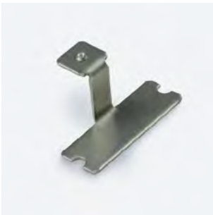
KKBK-06 Fixed bracket (allow 3 per metre/40in) S/Steel finish L20/W29.1/H28.8mm L0.79/W1.15/H1.13"
