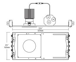
Mounting: IC Box / New Construction Chicago Plenum
