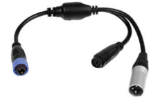
MLB-T-CONN-3P T Connector (IP67) 3-PIN XLR Male for DMX 4-PIN M15 Female for LED 2-PIN M15 Screw Lock Male for Power
