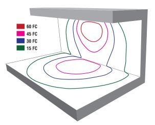
One 22" Edge provides ample illumination beneath a 4 ft. binder area. For additional output specify a 45" luminaire rather than two 22" luminaires.
