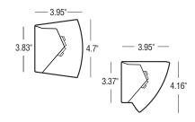
**DIMENSIONS AND LIGHT ENGINE** Extending less than 4" from the wall, Series 17 is ADA compliant and uses mid-powered LEDs yielding long life and even light distribution.
