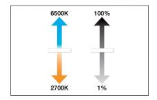
**TUNABLE WHITE** Any CCT between 2700K and 6500K with excellent CRI and R9 values; dimming from 100% to 1%.
