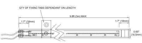
Micro LED strip fitted into 0.65" x 0.47" channel. Interior use only. Channel length up to 9.8ft (3m); strip comes in 1 inch (25mm) increments.
