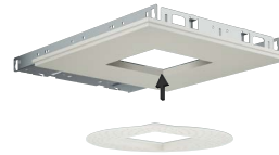
1. Fasten mud frame to ceiling.
