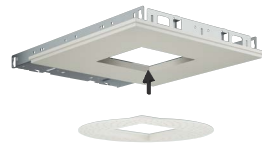
1. Fasten mud frame to ceiling.
