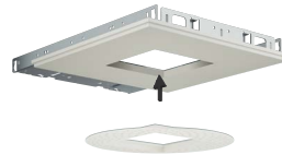
1. Fasten mud frame to ceiling.
