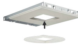
1. Fasten mud frame to ceiling.
