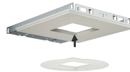
1. Fasten mud frame to ceiling.
