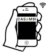
CASAMBI™ APP (IOS & Android) Wireless Commissioning, CCT & Light Intensity Control
