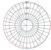
$Maximum\ Candela = 1841\ Located\ At\ Horizontal\ Angle = 0, Vertical\ Angle = 10$
