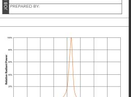
Dominant Wavelength Range Minimum Luminous Flux (lm) @ 350 mA Minimum Maximum Group DWL DWL Group Color Flux (lm) (nm) (nm) Group P4 80.6 Ρ3 73.9 P2 67.2 Amber A2 585 A3 595 N4 62 N3 56.8
