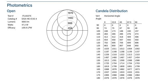
For all available IES files, please visit our website at pinnacle-ltg.com. Photometry testing in accordance to IESNA-LM-79-08 at an NVLAP accredited testing laboratory. Testing conducted at 25°C ambient conditions.
