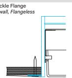
Recessed box allows for 1/2" of adjustability to accommodate a variety of grid ceilings
