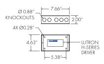
Remote power supply enclosure. 20.0 W Hi-lume Premier 0.1% EcoSystem w/Soft On, Fade to Black. Can power up to 2 single fixtures.
