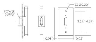
Optional cover plate provided allow mounting to single gang junction boxes at power feed location. Power supply to install in single gang junction box. Junction box provided by others. Cover plate finish same as fixture.
