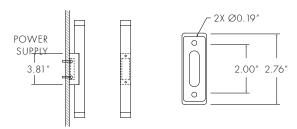
A low-profile back block that mounts directly to a wall to provide a clean and minimal look. For this configuration power supply must be installed remotely in a junction box or similar rated enclosure, and all splicing at fixture must be done in accordance with electrical code.
