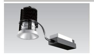
4-inch aperture high lumen recessed downlight utilizing Meteor Lighting's proprietary ColorFlip<sup>™</sup>W + RGB solution, that gives you True White light and unlimited RGB possibilities. This product is compatible with all DMX control systems and follows ANSI E1.20 RDM protocol. You can now get white and RGB colors all from a single light source.
